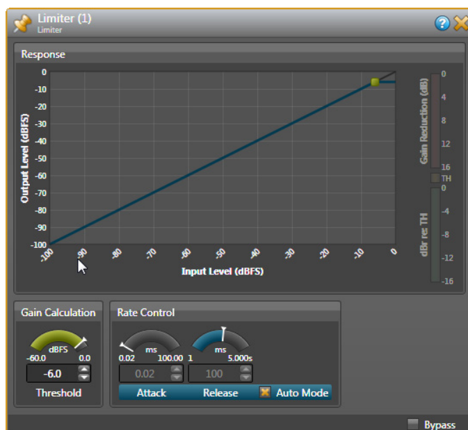
Figure 14c. Halogen Limiter control block.
